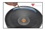
Step 10. – Using paint brush, apply a coat of dampening solution (white) to cone edge.
