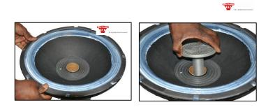
Step 11. – Glue gaskets in place to basket and line up with chassis holes. After glue has been cured, replace inner cooler.
